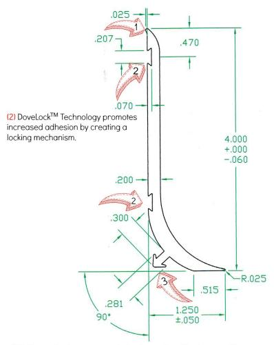
(3) Cove Anchor serves to both anchor the base of the cove to the floor and wall interface, and to lock-out moisture intrusion.
